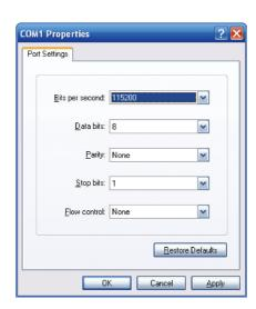
Figure 4-2: COM Port Configuration
