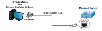
Figure 4-1: Managed Metro Switch Console Connectivity
